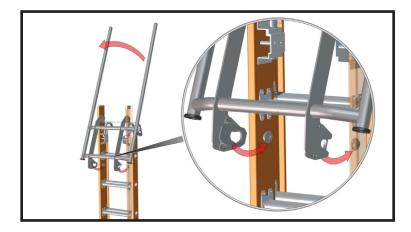
3. Swing the bottom of the bracket into the bottom posts until the latches engage onto the posts.
