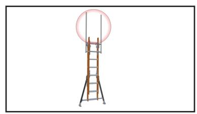
9. When you reach the top of the ladder, place both of your hands on the rails located on either side of the ladder, and walk through.
