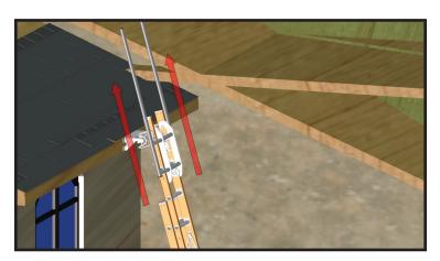
11. Lift up on the ladder to disengage the Claw from the (Ledge Lock).
