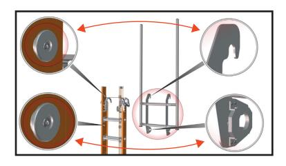
1. Make sure that the hooked ends of the Walkthrough brackets are lined up with the retention posts located on the inside of the ladder rails, and facing toward the climbing side of the ladder, as shown in the illustration.
