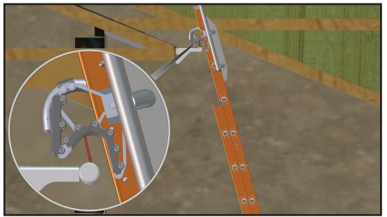
12. Once the ladder is free of the (Ledge Lock), you will be able to raise and lower the height of the ladder freely.
