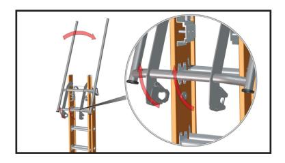
15. Swing the bottom of the bracket away from the ladder.
